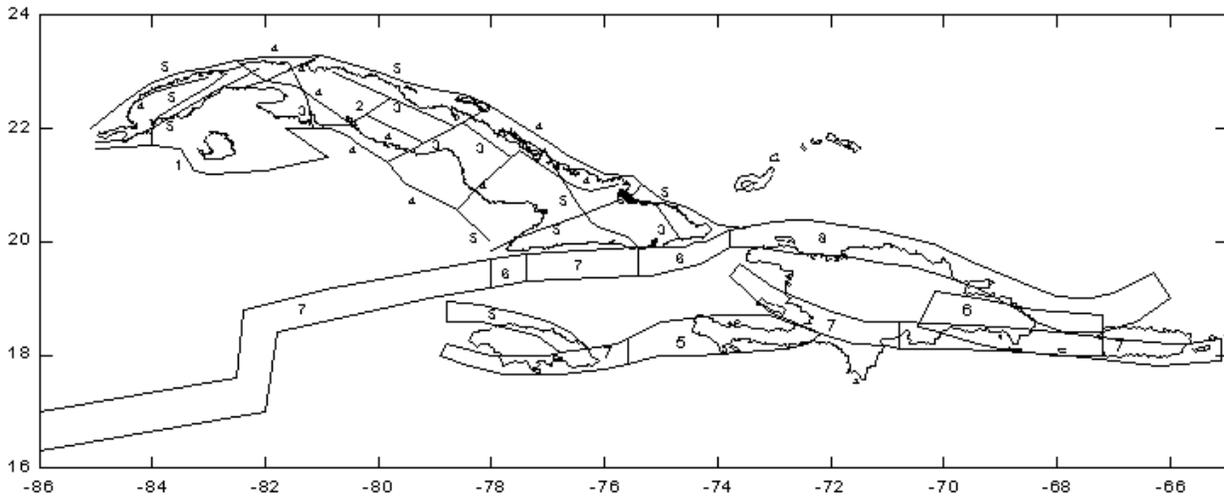
**Fig. 2.** Map of seismogenetic zones with  $M_{max}$  values [modified from Cotilla et al. (1996)]. The seismic source zones represented by lines in the Cuban Island are of 10 Km wide. 1.-  $4.5 < M_{max} \leq 5$ , 2.-  $5 < M_{max} \leq 5.5$ , 3.-  $5.5 < M_{max} \leq 6$ ; 4.-  $6 < M_{max} \leq 6.5$ ; 5.-  $6.5 < M_{max} \leq 7$ , 6.-  $7 < M_{max} \leq 7.5$ , 7.-  $7.5 < M_{max} \leq 8$ , 8.-  $8 < M_{max}$
